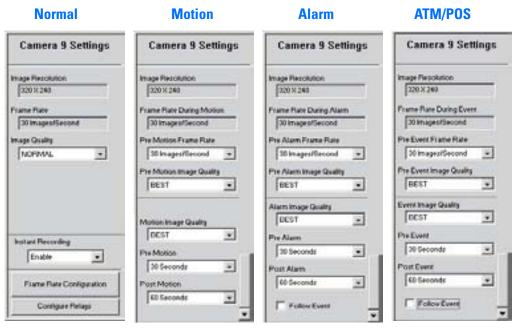
Figure 123. Examples of Custom Camera Settings
